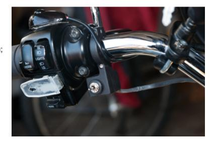
5. From the switch housing, route the wire harness along the handlebar past the inner fairing at the left fork tube to somewhere near the instruments.
