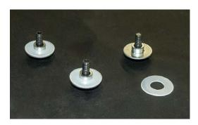
Windshield Flange Bolts and Nylon Washers Removed.
