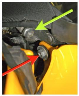
Windshield Garnish Bolt, Washer, Grommet (Red) and Windshield Clamp Nut (Green).
